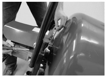
Use a Phillips screwdriver and 10mm wrench to tighten.
