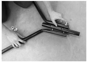
Put screws through corresponding mounting holes, attach two legs as shown. Note: Two legs have high mounting holes, and two have lower mounting holes.
