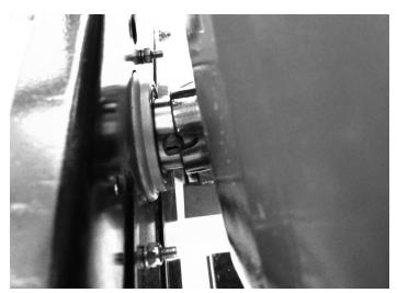
Drum will straddle set screw and fit tightly on motor spindle.
