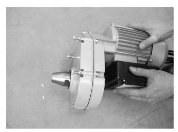
Remove nuts and washers from motor studs.
