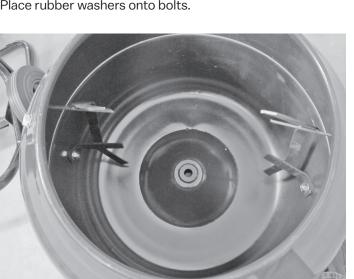
Fasten using a 19mm wrench and 19mm socket.
